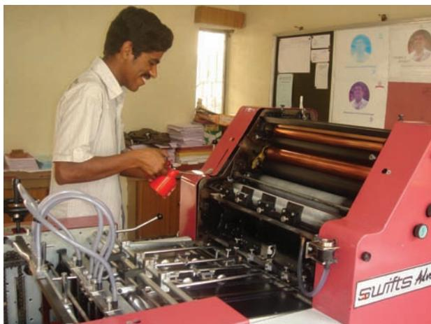
The mini offset printing machine, as a work station, caters to in-house requirements in smaller quantities
